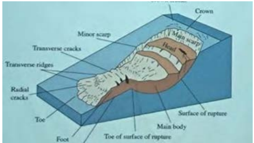
Anatomy of a Slope Failure ▲
