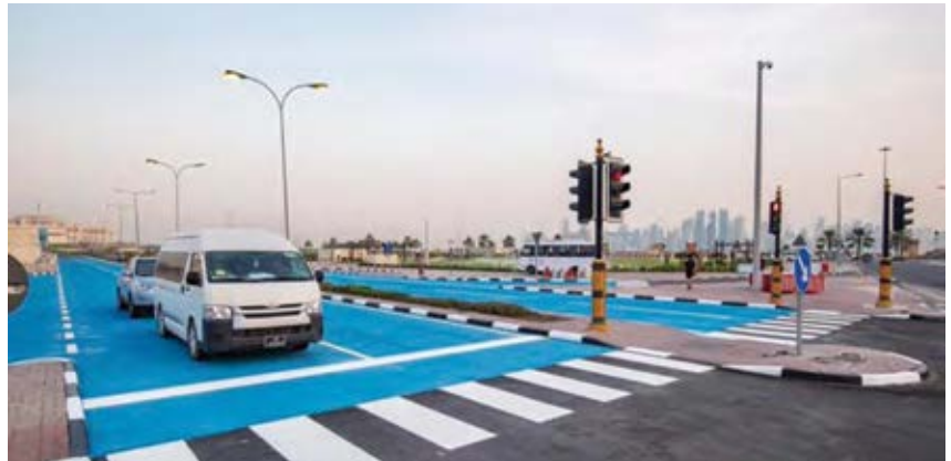
Doha engineers believe that painting asphalt will help reduce its temperature by 15-20 degrees, as well as increase the service life of the coating.
