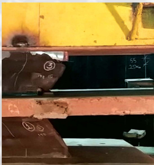
c. Failure in shear
